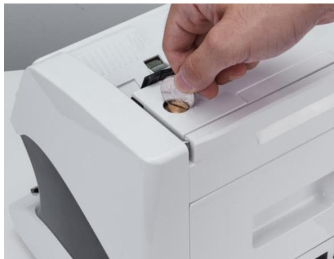
Figure 2-12 Using a coin to adjust the gap
